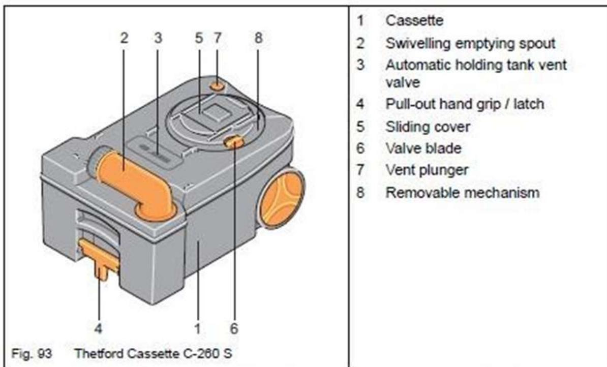
The cassette (Fig. 93/1) has a capacity of 18 l and should be emptied when the level indicator (Fig. 91/4) lights. Do not allow the cassette to become overfilled.
