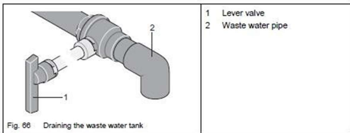
To empty the tank, you need to turn the lever valve to the right.
